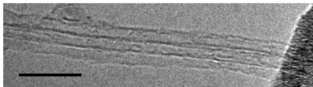
FIGURE 4. A TEM image of the PPEI-EI-SWNT sample on a holey LaCrO 3 stainless steel grid after thermal defunctionalization at 370 °C with air (scale bar = 10 nm). 23
